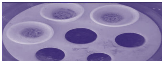
Figure 8. Banana fiber sample after moisture content test in a hot air oven
